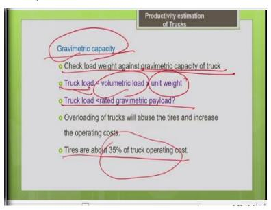
Another important thing you have to keep in mind is, for any machine whatever maybe the mission we have discussed about different types of machines so far. All the machines we are concerned about the safe gravimetric capacity of the machine. For every machine what is this safe operating load in terms of weight is given by the manufacturer, so that we call it as a gravimetric capacity.
