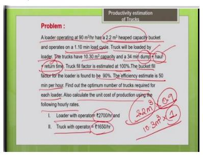
Now let us work on the problem on balancing the interdependent machines. So, here a loader is operating at 90-meter cube per hour and it has a 2.2 heap capacity bucket, and operates on 1.1-minute load cycle. The cycle time of the bucket is given as 1.1 minute, a cycle time per cycle it is 1.1 minute for the bucket of the loader. Truck will be loaded by the loader and the truck's capacity is 10.3-meter cube capacity and 34-minute dump + haul + return time.
