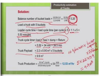
Now let us work out the solution, the first step will be to find the balance number of the bucket loads needed to fill the truck. How will you find the balance number of bucket loads needed to fill the truck? It depends upon your truck capacity and by your bucket capacity, so what is your truck capacity? It was given as 10.3-meter cube, you adjust it with the fill factor, truck fill factor is given as 1.
