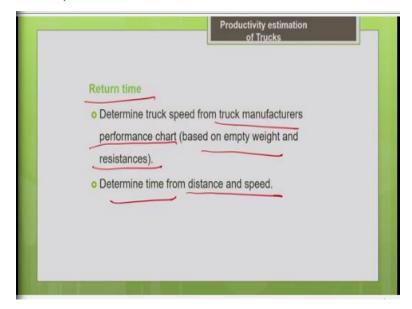
The return time the same way using truck manufacturer performance chart, but here the truck will be in the unloaded condition, empty weight, and consider the resistances also. So, you know the distance and speed I can calculate the return time, obviously the return speed will be more, so the return time will be less as the truck is in the empty condition.
