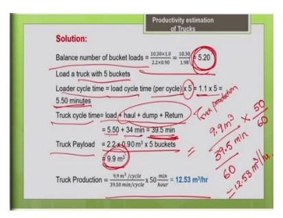
So, what is the volume of truck you are going to load in this case 9.9 meter cube, you are also supposed to check whether the truck payload is within the gravimetric capacity. If say gravimetric capacity is given by the manufacturer you have to check whether the weight of the load of material in the truck is within the gravimetric capacity. For that you need the input data of the density of the material also.
