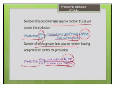
Now let us consider the case say the number of trucks lower than the balance number. Say I am going to round it to lower number, say I got 7.4 now I am going to round it to 7. When I round it to lower than the balanced number that means trucks are less than what is needed. So, trucks are more critical for the production, so here the loader will have the idle time, loader will be waiting for the truck, so truck cycle time will control the productivity of this stream.
